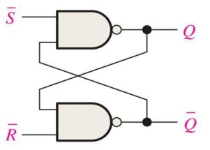
(b) Active-LOW input  $\overline{S}-\overline{R}$  latch
